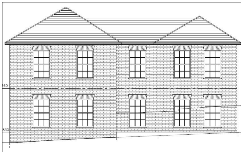
Fig. 4. Front elevation of existing building fronting St Albans Road (with proposed extension) as proposed under current application.
